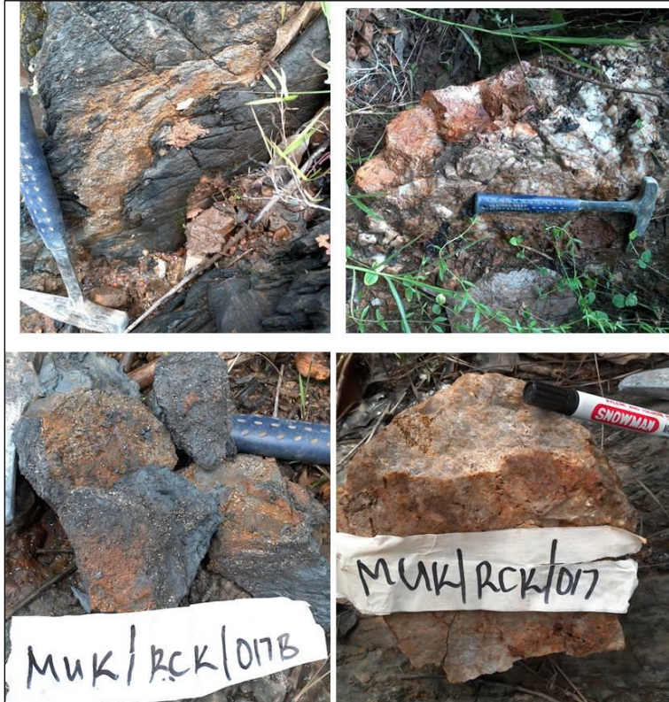
Figure 2: MUK/RCK is graphitic schist with massive sulphide along bedding planes. MUK/RCK/17B is quartz veins with sulphides. 824943mE/9840255mN
