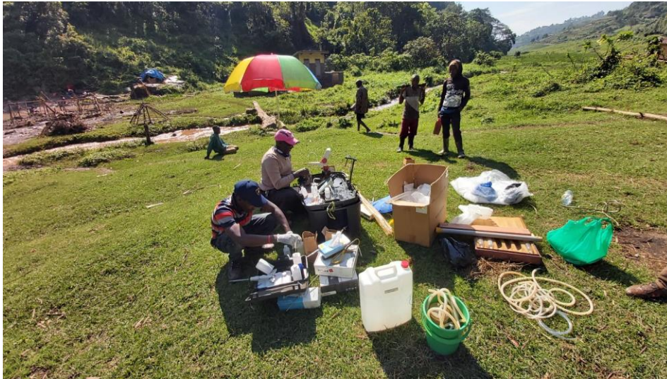
Figure 17: Analysis of volatile components of geothermal water at Karungu hot springs, Rubanda District.
