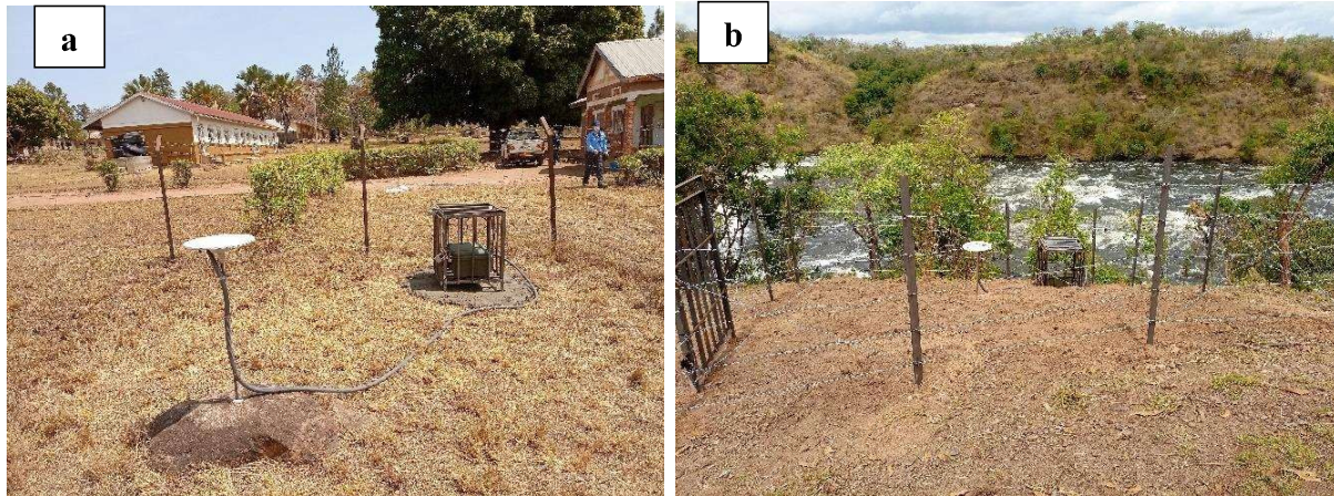
Figure 3: . (a) GNSS observation station was restored at Nakasongola site. (b) GNSS Observation Station installed at Top of the Fall, Murchison Falls Conservation Area.
