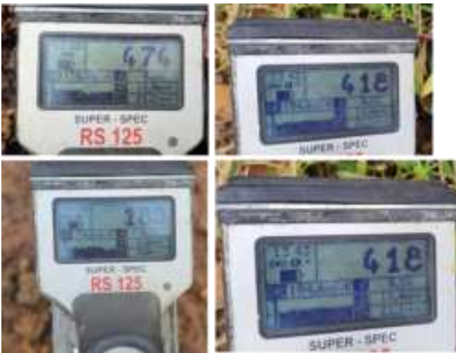
Figure 3: Radiation readings captured at the observation points in block 2 anomaly 2 Nakaseke District.
